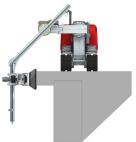
// EXTENDED OUTSIDE Allows for extended vertical operation as well as outside a Parapet beam.
