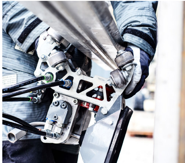
Roller beam have a light weight aluminum core and replaceable gear rack and guide rails. The Ergo Power Head is connected to the roller beam with a single bolt.
