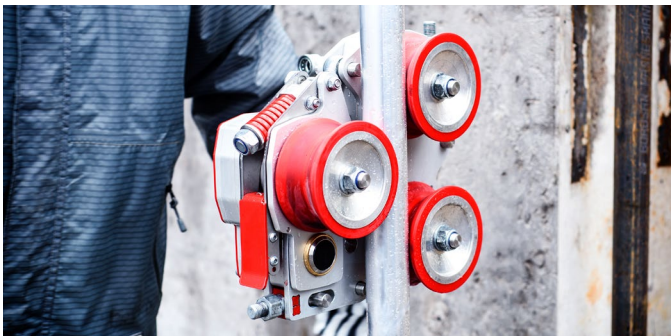
Climbers are fitted to the pipe by a single spring loaded handle
